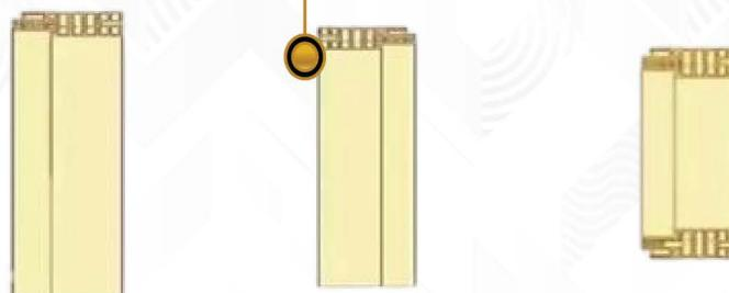
First, cut the door frame into 45° bevel
